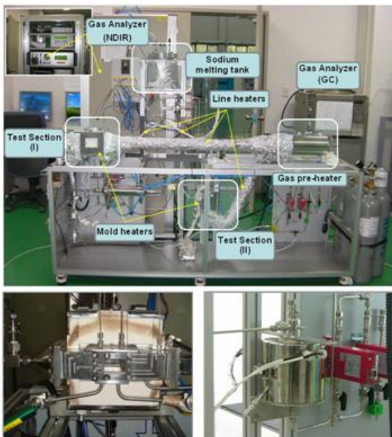
Figure 6: KAERI Sodium-CO 2 Reaction Test Facility
