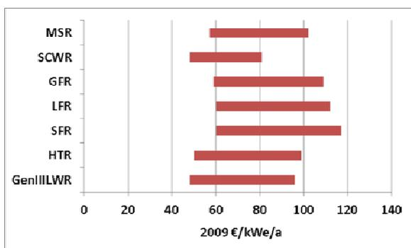
**Figure 7: Front-end fuel cycle cost ranges**
