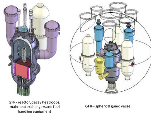
GFR - reactor, decay heat loops, main heat exchangers and fuel handling equipment
