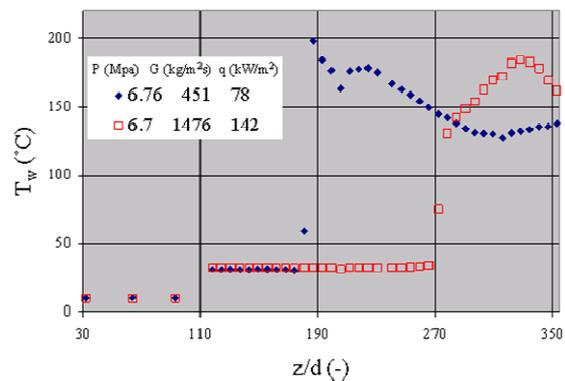
**Figure 7: Wall-temperature measurements at supercritical pressures in an 8 mm tube with carbon dioxide flow**
