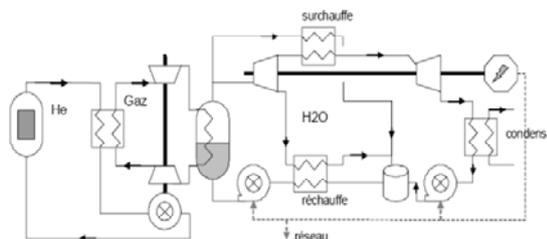
This option includes numerous assets, with at first the advantage to eliminate by design some of the loss of flow accidents which is particularly interesting for GFR safety demonstration. The attractiveness in terms of passiveness and autonomy is important: the main loops, by their natural adaptations to the primary thermal-hydraulic conditions, could be valued for long term core cooling either for pressurised or depressurised situation.
