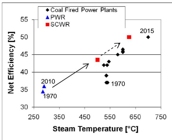
As sketched in Figure 1, the idea of the SCWR follows the trend of coal fired power plants within the last 40 years, which succeeded to increase the net efficiency while decreasing the specific capital cost by increasing the live steam temperature and pressure. Since about 1990, these power plants have usually been designed for supercritical steam conditions, reaching up to 50% efficiency in the near future, whereas water-cooled reactors are still built with similar parameters as in 1970.
