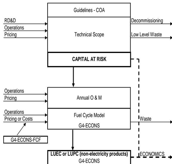
The central feature of the methodology is the comprehensive Code of Accounts. The Code of Accounts (COA) provides a disciplined structure for capturing and categorizing all appropriate costs in the development of a consistent system cost estimate.
