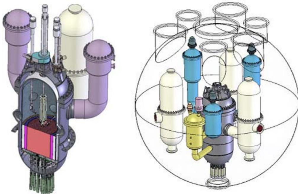
GFR - reactor, decay heat loops, main heat exchangers and fuel handling equipment
