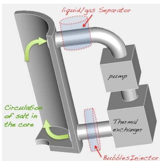
Figure 3-25: FFFER Molten Salt Loop Design, without Instrumentation, Heating, Insulation and Gas Supply
