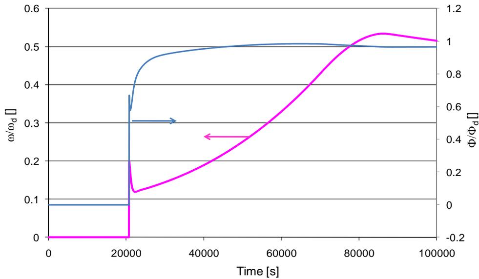
Furthermore, it can be seen on Figure 3-16 that the machine start-up with the motor leads to a peak in the mass flow rate, which then stabilizes at about 40 kg/s. This mass flow peak translates into a temporary decrease of fuel temperature, which then goes up again to stabilize below a still convenient value of 1 000°C, i.e. much below the Category 4 accident limit of 1 600°C (Figure 3-17).
