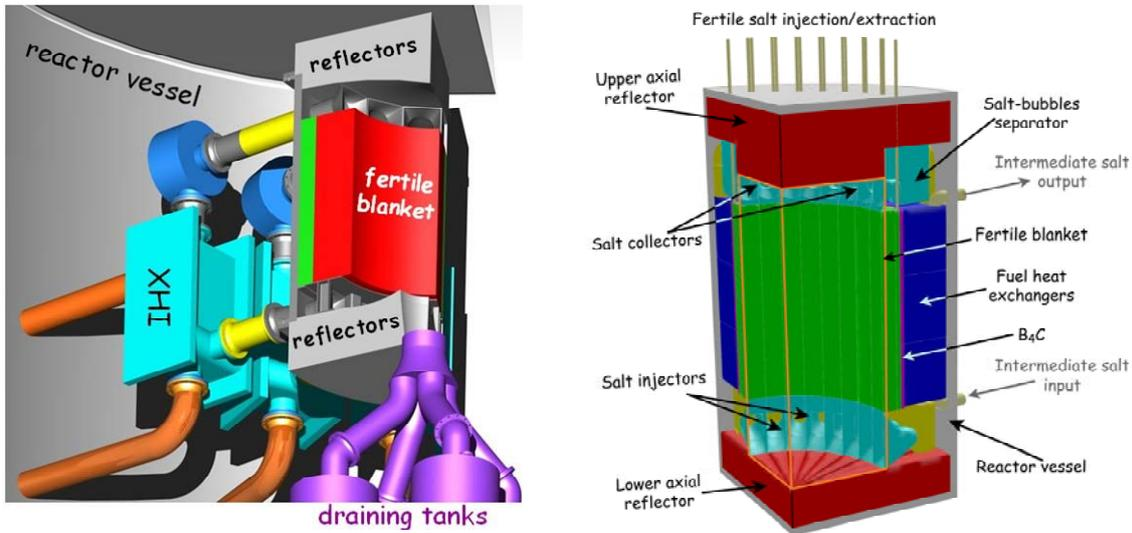
In the MSFR, the liquid fuel processing is part of the reactor where a small side stream of the molten salt is processed for fission product removal and then returned to the reactor. Because of this design characteristic compared to classical solid-fuel reactors, the MSFR can therefore operate with widely varying fuel compositions.
