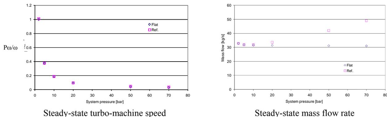
Finally, CATHARE simulations have been performed for complete DHR scenarios for the GFR, involving loss-of-coolant-accidents (LOCAs) in conjunction with loss of back-up-pressure (LOBP). Thereby, it has been shown that, in each of the investigated cases, incorporation of the Brayton-loop turbo-machine with nitrogen indeed leads to fuel temperatures remaining considerably below Category 4 accident limits of 1 600°C.
