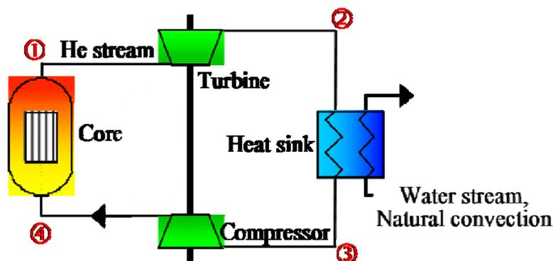
An analytical model based on simplified thermodynamic and aerodynamic equations was developed to highlight design choices. Two different machine designs are analyzed: a Brayton-loop turbo-machine working with helium, and a second one working with nitrogen, since nitrogen is the heavy gas foreseen to be injected into the primary system to enhance the natural convection under loss-of-coolant-accident (LOCA) conditions.
