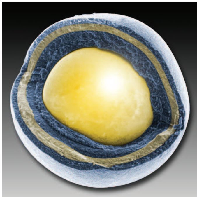
Left: Next-generation TRISO fuel particles have several layers of carbon and silicon carbide that serve as the primary containment for radioactive material. Right: A cross-section of a fuel pellet containing TRISO particles.
