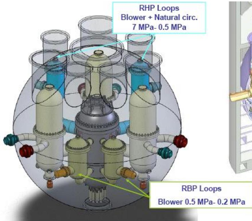
Figure 2: GFR Primary and DHR system inside the guard containment
