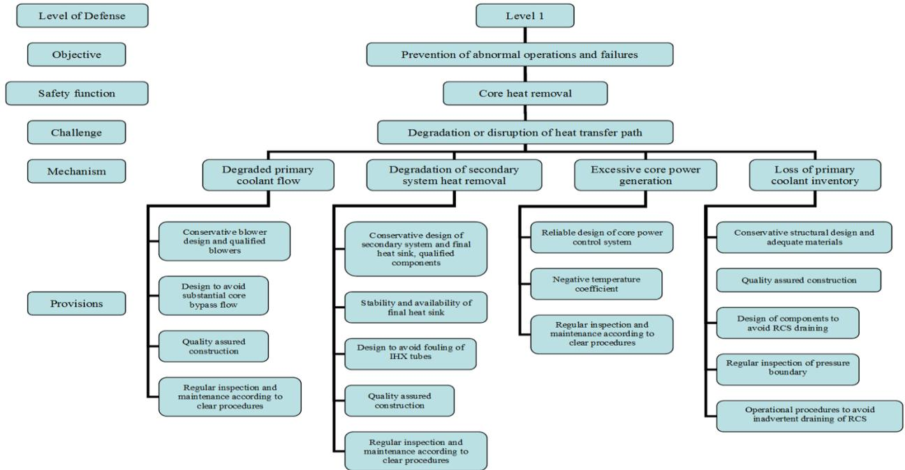
Figure 5: ALLEGRO OPT for Level 1 of DiD, heat removal from the core
