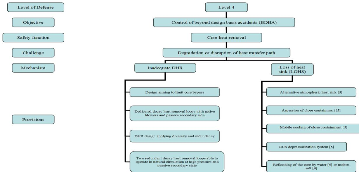
Figure 8: ALLEGRO OPT for Level 4 of DiD, heat removal from the core
