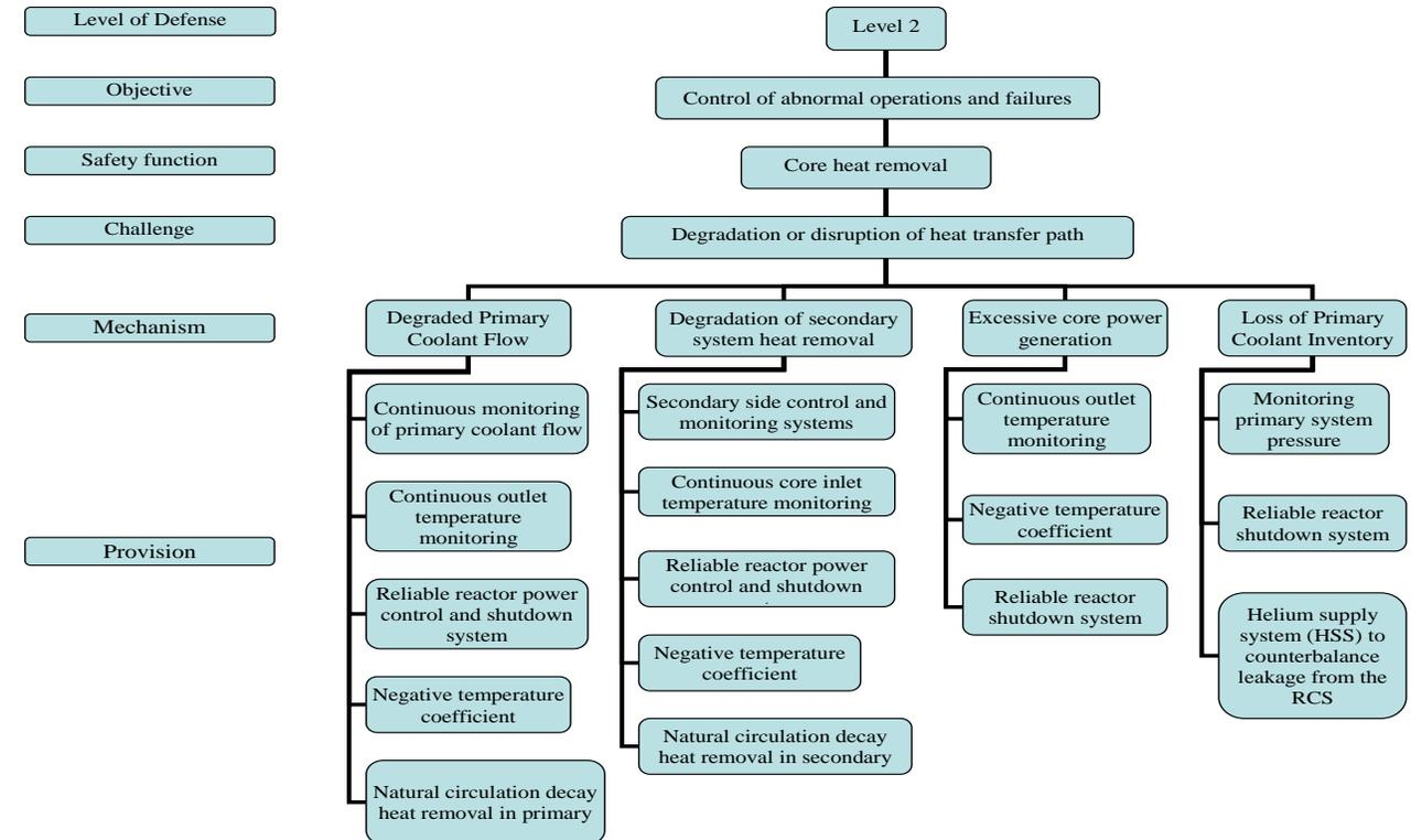
Figure 6: ALLEGRO OPT for Level 2 of DiD, heat removal from the core
