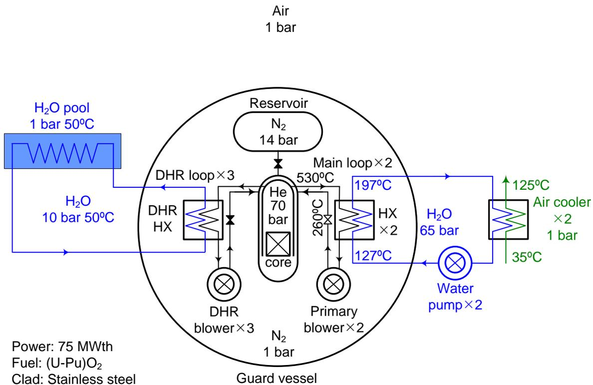
Figure 4: A simplified diagram of the ALLEGRO gas-cooled fast reactor
