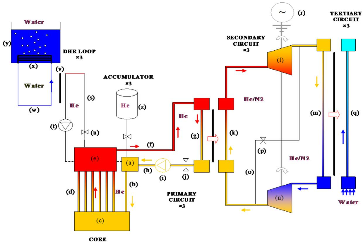
Figure 9: GFR system nodalisation diagram
