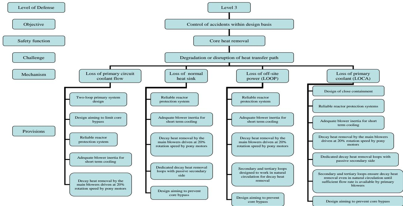
Figure 7: ALLEGRO OPT for Level 3 of DiD, heat removal from the core
