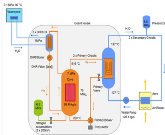
**Figure GFR 2. The GFR core concept**
