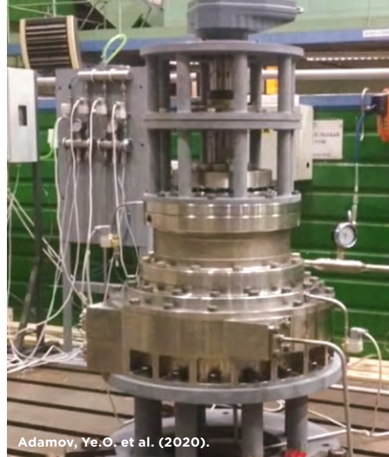
Figure LFR-3: Testing of the friction pair of the MCP lower radial bearing as part of the model block
