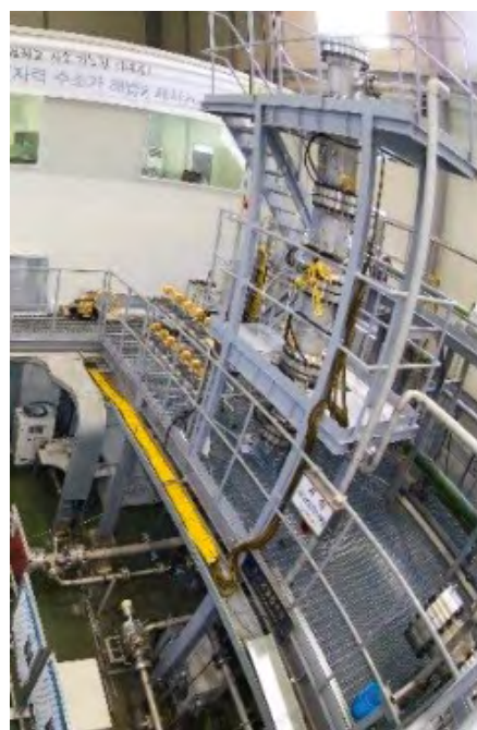
Figure VHTR-11. Component scale helium gas loop
