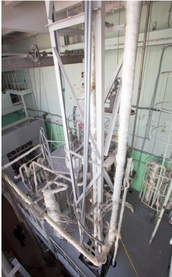
The experiments were performed with a single-tube model at the “SPRUT” test facility with the aim to justify the design parameters of a new design of a large-modular reactor steam generator where within one shell the processes of steam evaporation and superheating take place, at the modes of 12.5% and 75% of the nominal sodium flow rate, with real parameters in the sodium loop and high-pressure water loop.
