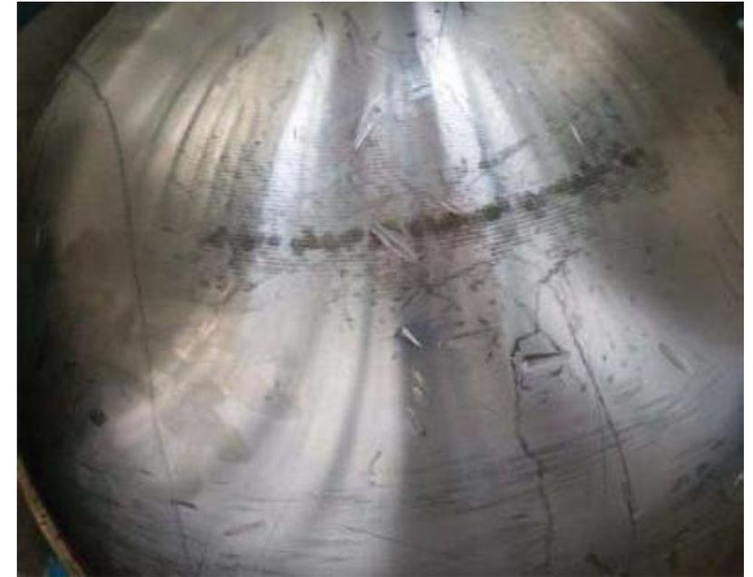
Check valve (sphere) after endurance tests
