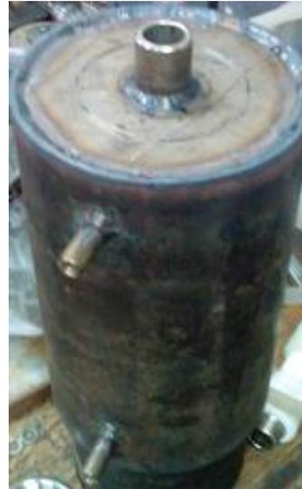
Getter purification module, 6 kg of zirconium powder
