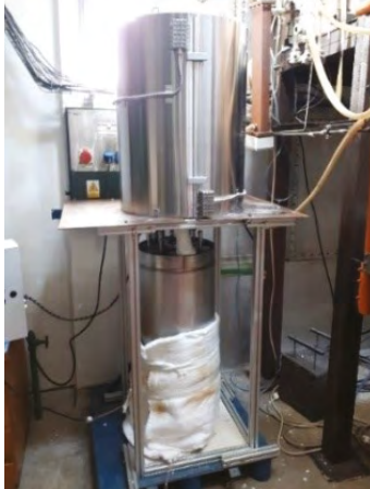
Figure MSR-3. Pouring the FLIBE melt into the central container of the zone and checking the complete zone in the LR-0 reactor vessel
