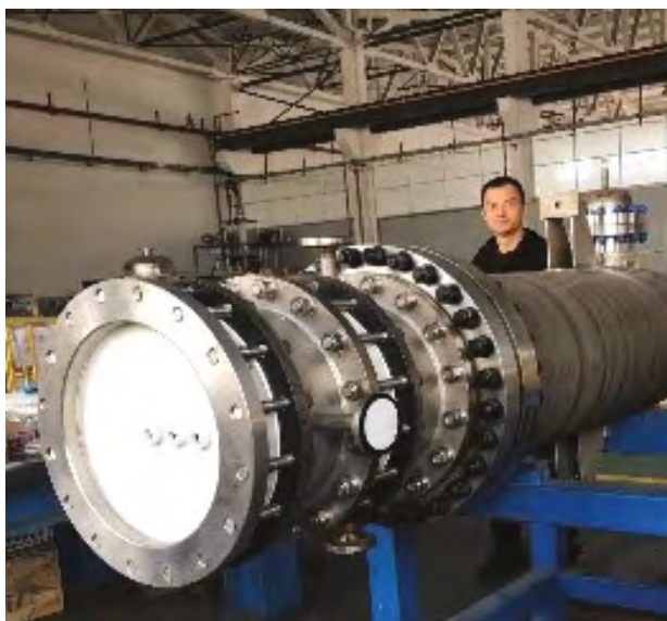
Figure VHTR-6: Prototype of the sulfuric acid decomposer
