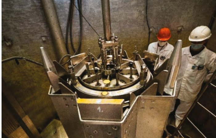
Figure MSR-3. Pouring the FLIBE melt into the central container of the zone and checking the complete zone in the LR-0 reactor vessel
