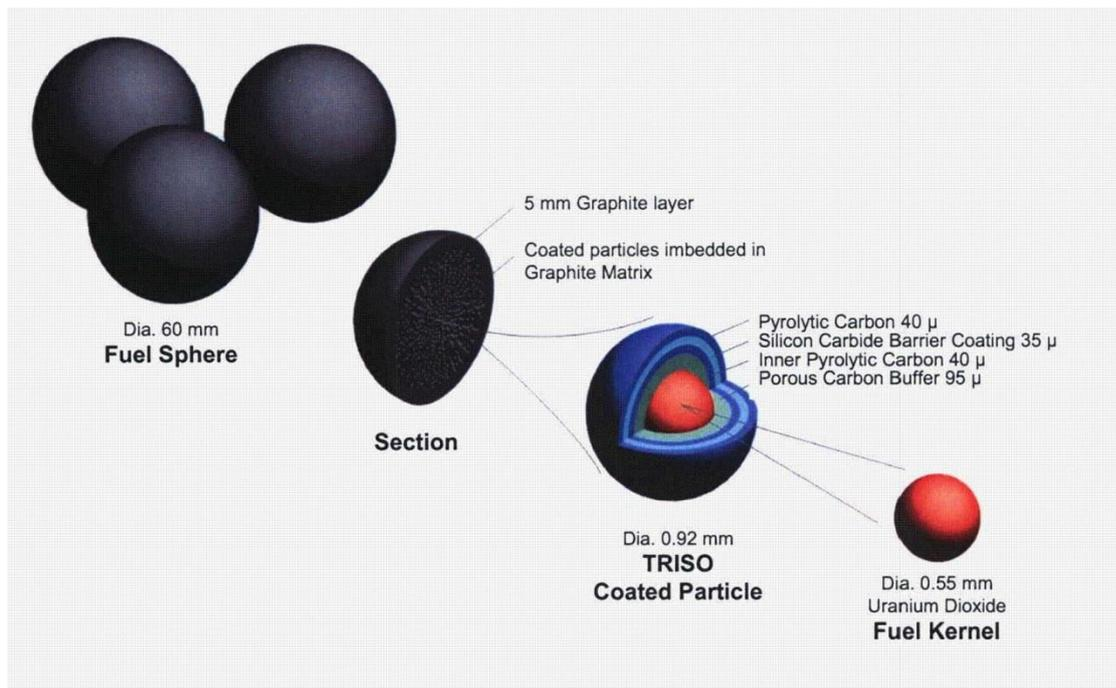
Figure 4: Illustration of Coated Particle Fuel in Pebble Fuel Element [2, 15].
