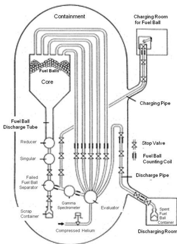
Figure 14: Movement of the fuel pebbles for P-VHTR [15,28].
