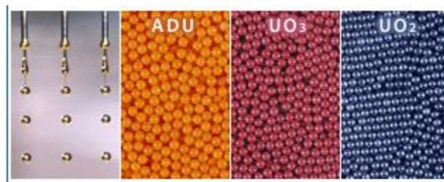
Figure 10: Fuel kernel fabrication through dropping uranyl nitrate stock solution [24].
