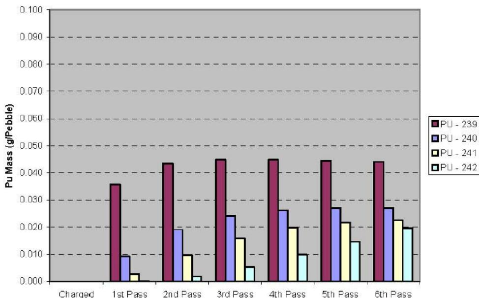
Figure 15: Plutonium build-up in a PBMR fuel element in an equilibrium core [14].
