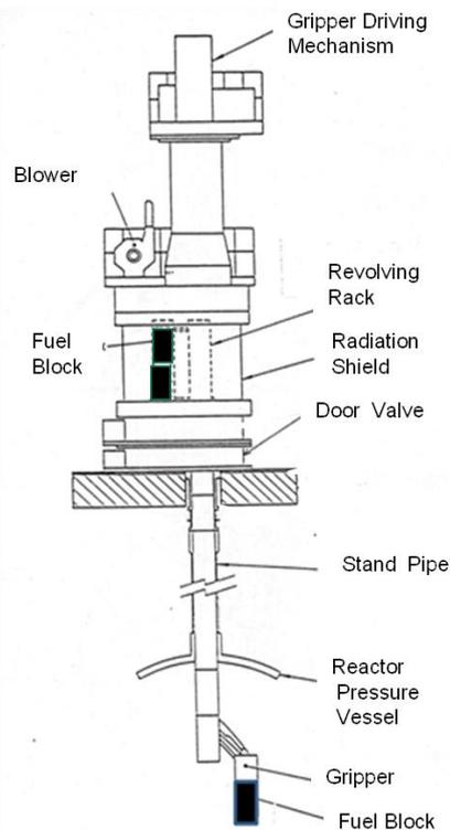
Figure 12: Door valve and refueling machine [27].
