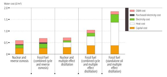
Figure 6: Cost of desalinated water by fuel and process
