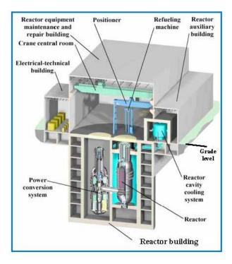
Figure 3: GT-MHR Fully-Embedded Reactor Building [2].
