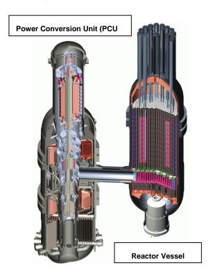
Figure 2: GT-MHR Reactor, Cross-Duct and PCU Vessels [2].
