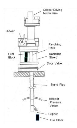
Figure 12: Door valve and refueling machine [27].
