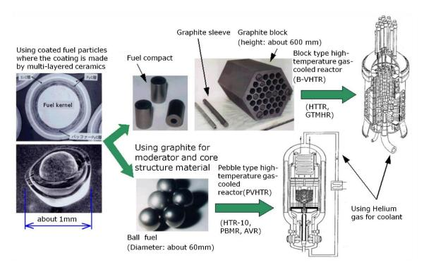
Figure 7: B-VHTR and P-VHTR as well as their fuel elements.
