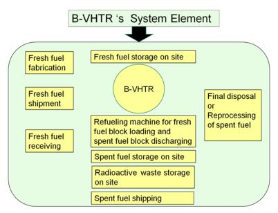
Figure 8: B-VHTR System element.
