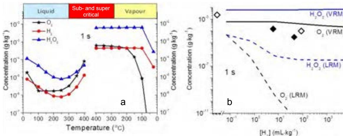
(a) Effect of H<sub>2</sub> addition on the concentration of oxidising species predicted by the models. (b) Symbols represent plant data from Beloyarsk NPP, which operated with nuclear steam reheat (open symbols: H<sub>2</sub> produced by radiolytic decomposition of NH<sub>3</sub>, solid symbols: direct H<sub>2</sub> addition).
