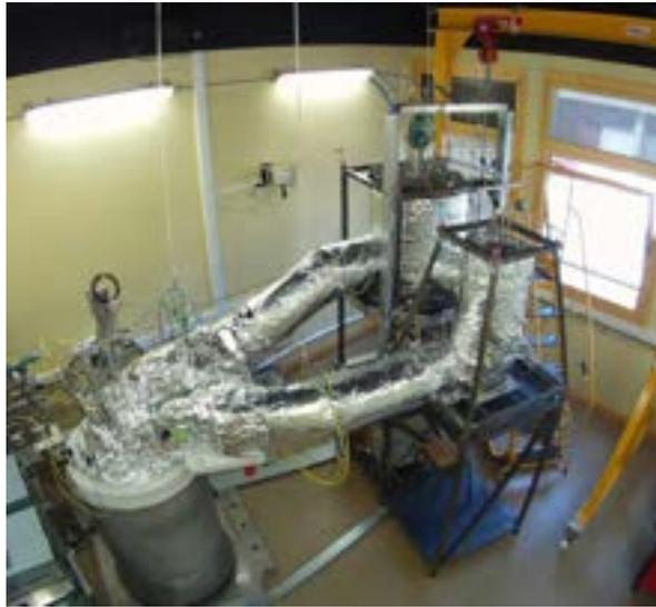
Figure 3.46: **UC Berkeley Compact Integral Effects Test Facility. The facility uses a simulant fluid (DowTherm A) to enable experimental evaluation of liquid salt thermal and hydraulic performance**
