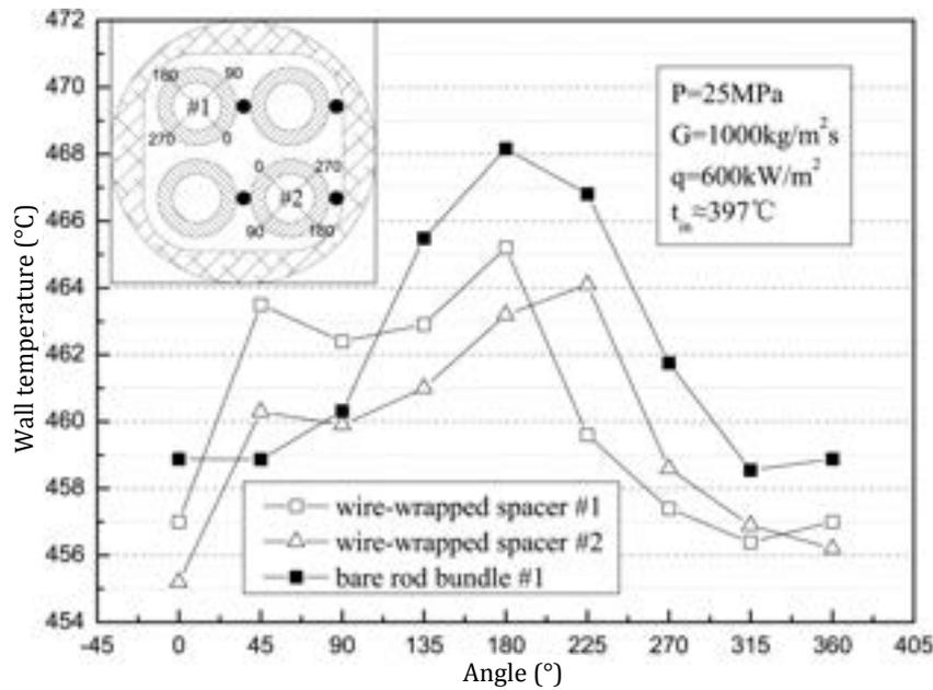
Figure 3.20: **Circumferential temperature maps obtained with the 3-rod bundle cooled with CO<sub>2</sub> flow**
