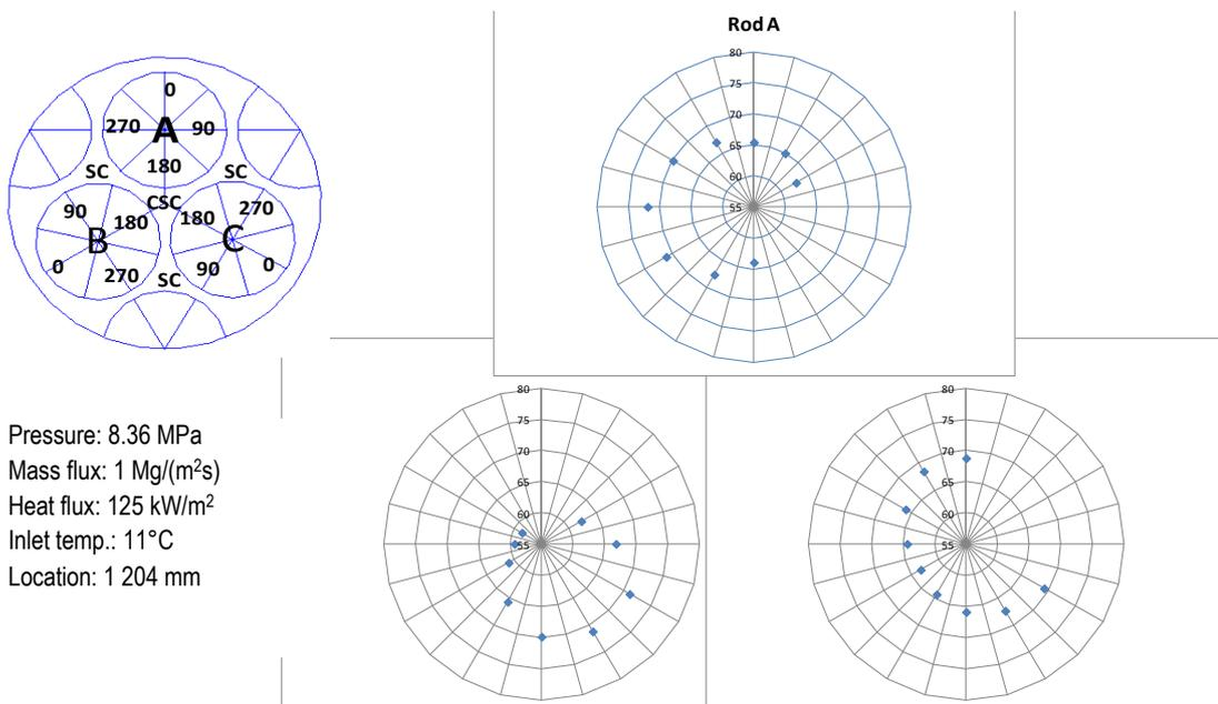
Figure 3.21 illustrates the axial surface temperature measurements at the peak temperature angle of each rod. Some fluctuations in surface temperature have been observed mainly due to the presence of the wire-wrapped spacer. It appears that no significant increases in wall temperature (corresponding to the deteriorated heat transfer phenomenon) were encountered over the heated rod. As indicated above, there are insufficient data to confirm the peak-
