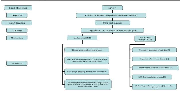
Figure 8: ALLEGRO OPT for Level 4 of DiD, heat removal from the core
