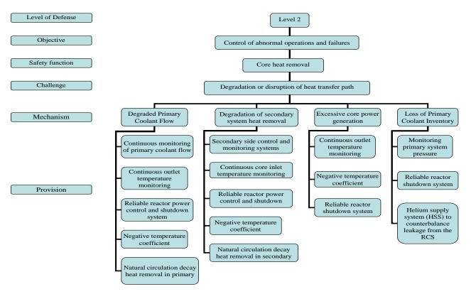
Figure 6: ALLEGRO OPT for Level 2 of DiD, heat removal from the core
