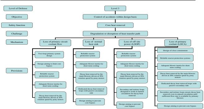
Figure 7: ALLEGRO OPT for Level 3 of DiD, heat removal from the core
