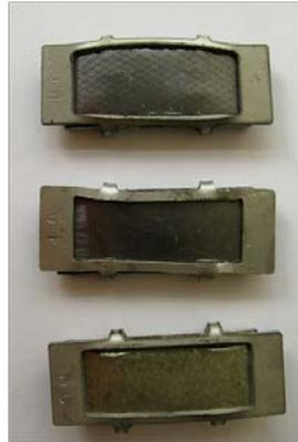
Figure 3.56: Graphite sealing after exposure
