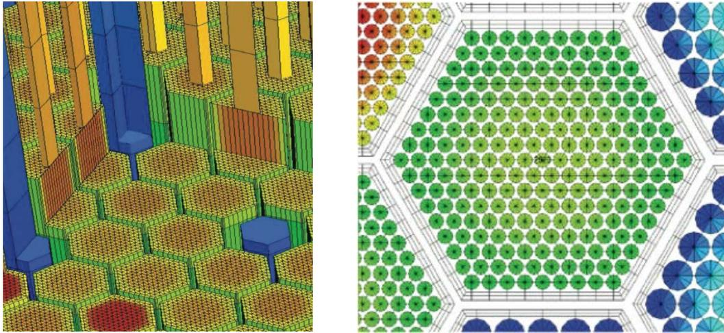
CATHARE can be used to model a complete experimental loop or reactor circuit with a 1D representation of the test section; this model may be replaced with a Trio\_U MC model of the test section itself in order to account for 3D boiling effects. In the case of the 6-equations CATHARE code, the applicability of its current closure laws to two-phase sodium flow must be evaluated; for the 3-equations MC code, new numerical methods are needed as well.
