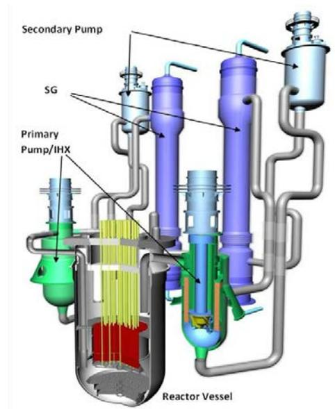
Figure 3.58: **Example sodium fast reactor (pool-configuration SFR)**
