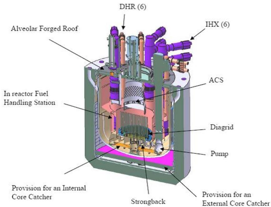
Figure 3.59: **Korea advanced liquid metal reactor (pool-configuration SFR)**
