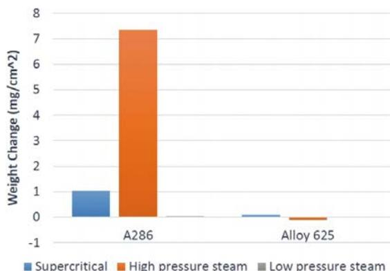
Figure 3.43: Weight change as a function of exposure time in SHS
