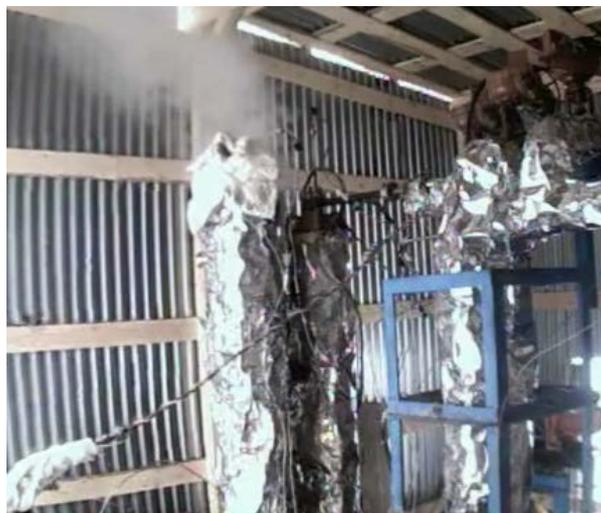
The reactor main coolant pump is intended to establish the lead coolant head and provide for its circulation in the circuit. To confirm its serviceability, several mock-ups of the pump set have been developed, as well as the test sections to check their performance:
