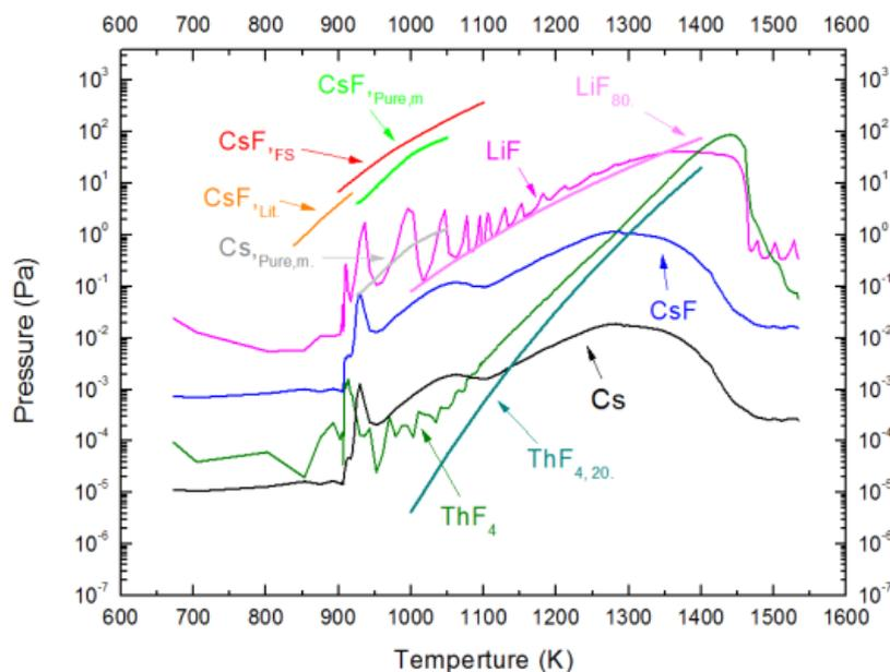
Note: Blue and black lines are the partial vapour pressures of gaseous  $\text{CsF}$ , resp.  $\text{Cs}$  gaseous species in equilibrium with condensed  $\text{CsF}$ , while light green line corresponds to measurement of pure  $\text{CsF}$ , indicating much higher volatility compared to dissolved  $\text{CsF}$ .
