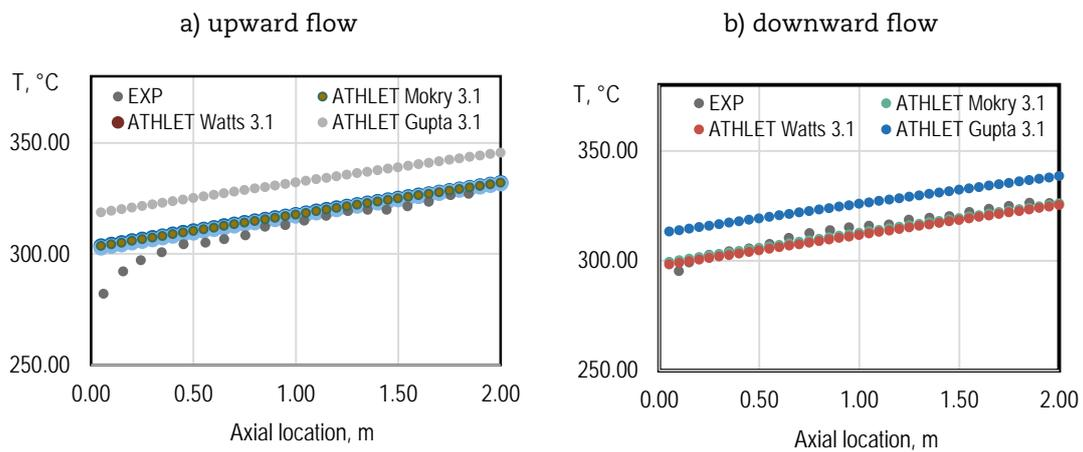
Figure 3.40: Bulk temperature distribution
