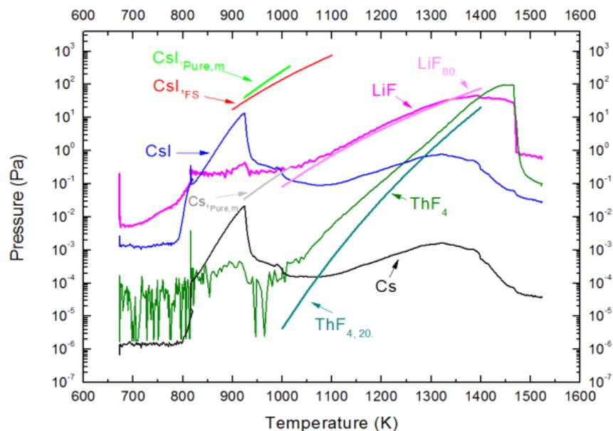
Blue and black lines are the partial vapour pressures of gaseous CsF, resp. Cs gaseous species in equilibrium with condensed CsF, while light green line corresponds to measurement of pure CsF, indicating much similar volatility compared to CsF in the mixture, demonstrating its reluctance to dissolve in the fuel matrix.
