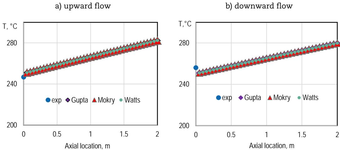
Figure 3.39: Wall temperature distribution for Case 2 Variant 1
