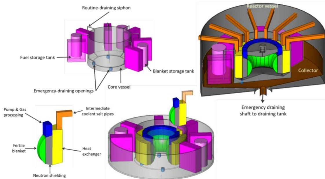
Each sector comprises: a heat exchanger, a circulation pump, a bubble injector and a gas separator, a blanket salt tank, and a heat exchanger (Figure 3.9, bottom left). Each sector is connected to an intermediate fluid circuit (four circuits, each feeding four sectors, for example).
