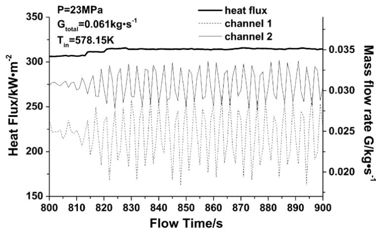
Figure 3.30: Effect of flow direction on heat transfer at supercritical pressures
