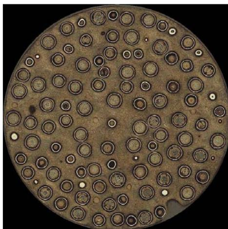
The PIE of High-Flux Reactor (HFR)-EU-1 containing Chinese and German fuel irradiated at typical pebble-bed conditions is also completed.
