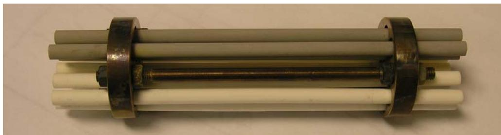
Figure 3.55: Graphite sealing before exposure
