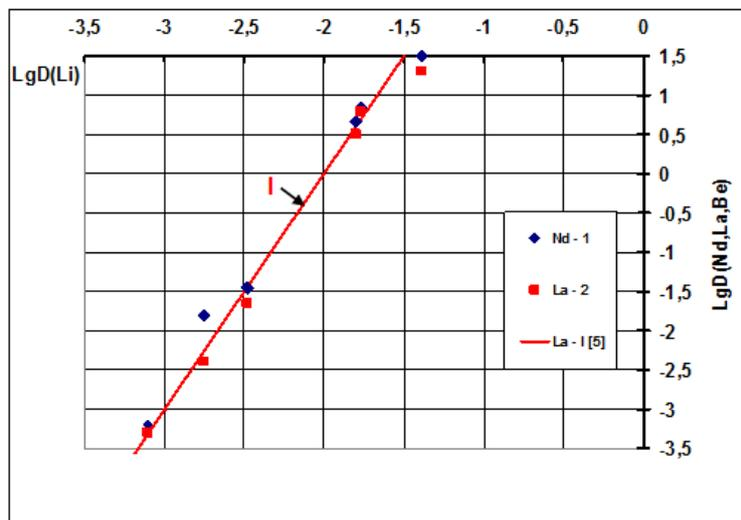
The valences of lanthanum and neodymium in the molten  $73LiF-27BeF_2$  salt mixture are 3. Neodymium is extracted more effectively compared to lanthanum. The separation factor is  $\alpha = D(Nd)/D(La) = 1.58-1.60$ . It should be mentioned that unlike Nd and La, Be is not practically extracted into bismuth from melt  $73LiF-27BeF_2$  and its distribution coefficient makes up  $D(Be) < 0.003$  if  $D(Li) < 0.04$ .
