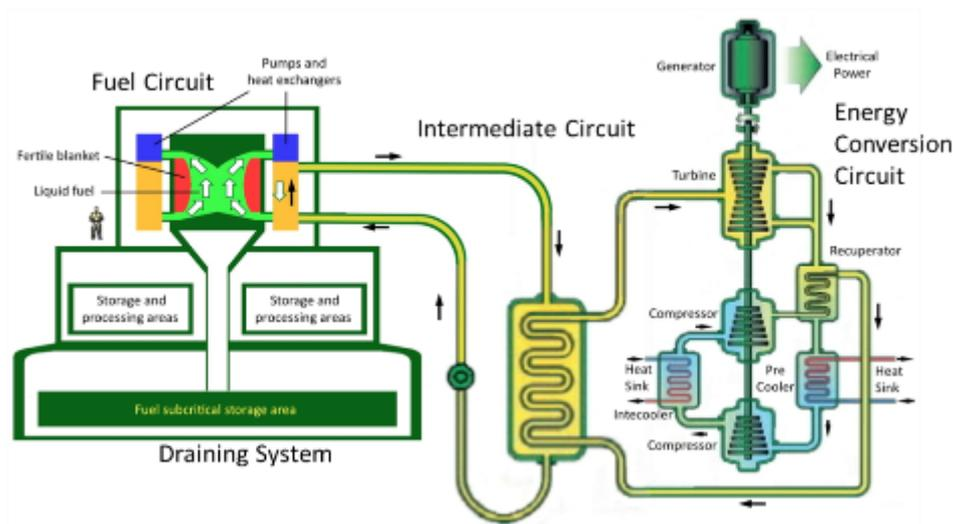
The fuel circuit (see Figure 3.6 – left), defined as the circuit containing the fuel salt during power generation, includes the core cavity and the recirculation loops (also called “sectors” in the following) comprising the inlet and outlet pipes, a gas injection system, salt-bubble separators, pumps and fuel heat exchangers (Brovchenko et al., 2014). The dimensions of the core cavity are given in Figure 3.8 (middle and right); (Laureau, 2015a; Rouch et al., 2014).
