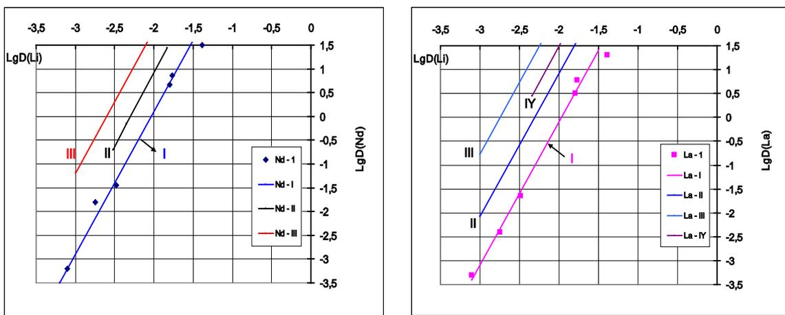
**Left:** I – current work; II – (Ferris, 1970; Ferris, 1971) for  $66.7\text{LiF}-33.3\text{BeF}_2$  eq.  $\lg D(\text{Nd}) = 3\lg D(\text{Li}) + 7.806$ ; III – (Grimes, 1970) for  $66\text{LiF}-34\text{BeF}_2$  eq.  $\lg D(\text{Nd}) \approx 3\lg D(\text{Li}) + 7.45$
