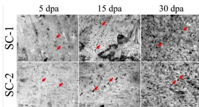
Figure SCWR 11. The density of defects obtained by TEM of ally SC1 and SC2 irradiated at 550°C
