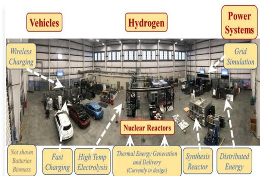
**Figure VHTR 8. 25 kW HTSE Test Facility in DETAIL within the INL Energy Systems Laboratory**
