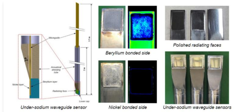
JAEA developed an improved imaging under sodium viewer for a middle distance (see Figure SFR.9). The transmission sensor provided better profile of the wave, and the receiving sensor successfully reduced the noise of the wave profile. The imaging experiment in water showed that higher resolution can be obtained through the improvement of the imaging under sodium viewer.
