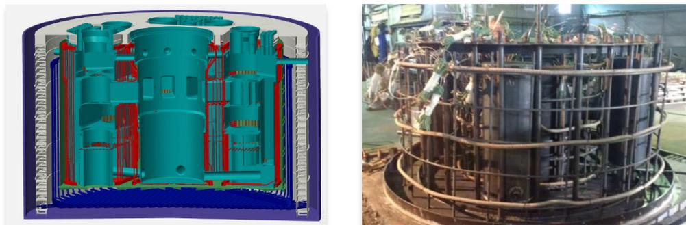
The BREST-OD-300 has a submerged-type once-through steam generator with a coiled heat exchanger. Silicon-containing austenite steel is used as the material of the heat-exchange tubes. Experiments were conducted to study the dependent failure of tubes caused by the rupture of one tube. The results of the experiments in lead coolant conditions simulating full-scale ones (temperature, pressure) have shown no dependent failure. Serviceability of the assembly for the
