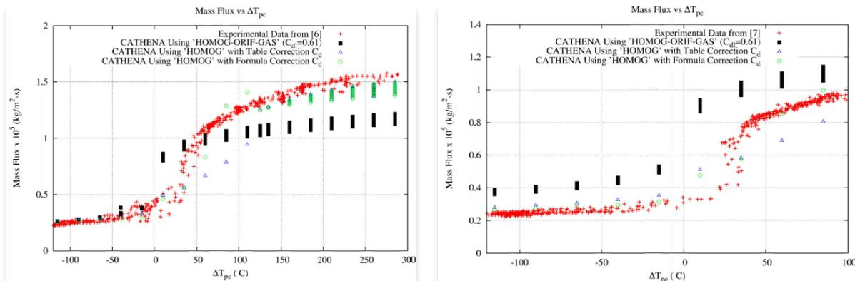
Figure SCWR4. **CATHENA Mass Flow Rate Predictions of Two Parallel Channel Instability (Left). CATHENA Predicted Velocities and Pressure Drops in a Natural Circulation Loop (Right)**
