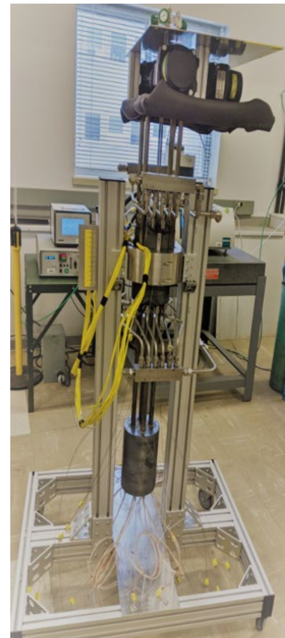
Assembled and instrumented array sodium heat pipe 50
