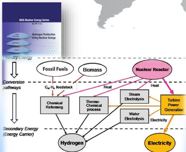
FIG. 8. Nuclear hydrogen cogeneration routes.
