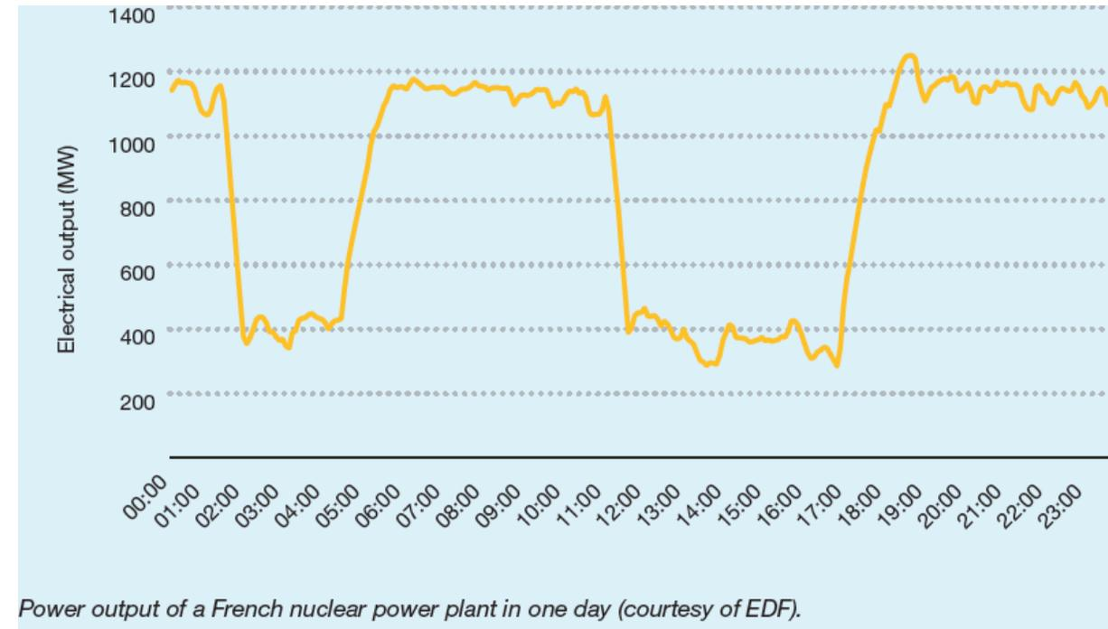
Power output of a French nuclear power plant in one day (courtesy of EDF).
