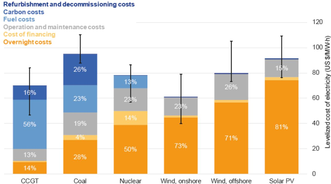
*FIG. 8. Median values for the LCOE generation for different technologies, assuming a discount rate of 7% and carbon cost of US \$30/tonne, with error bars representing the first and third quartiles for the lower and upper bounds, respectively. Source: Ref. [53]. Note: MW·h — megawatt-hour.*
