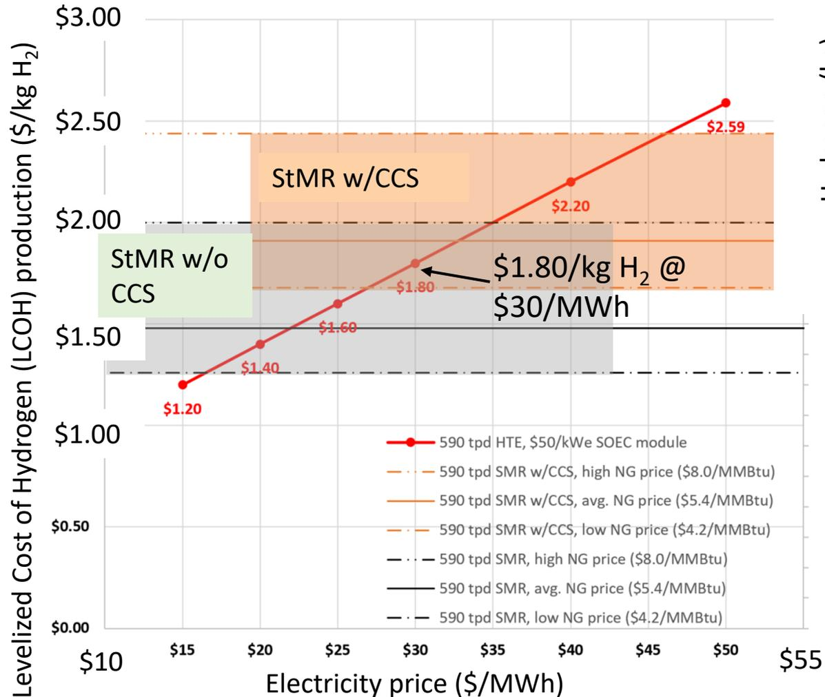
LWR-HTSE LCOH as a function of electricity price compared to the Steam Methane Reforming (StMR) plant (with and without carbon capture and sequestration [CCS]) LCOH with low, baseline, and high natural gas pricing.
