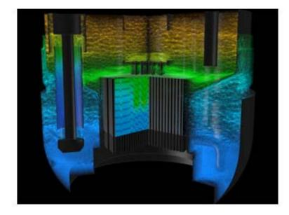
Modelling of an accidental scenario with loss of the primary pump of ASTRID reactor, without control rod protection (ULOF). Natural convection is leading to a stabilised sodium flow in te core allowing core assemblies cooling and avoiding a severe accident situation (no core or fuel melting). CEA/Saclay studies
