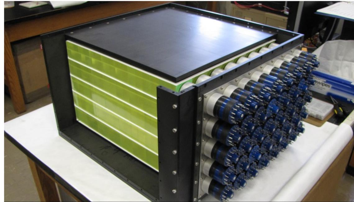
The MiniCHANDLER Prototype, open during assembly to show the cubes and  ${}^6\text{Li}$ -doped ZnS sheets
