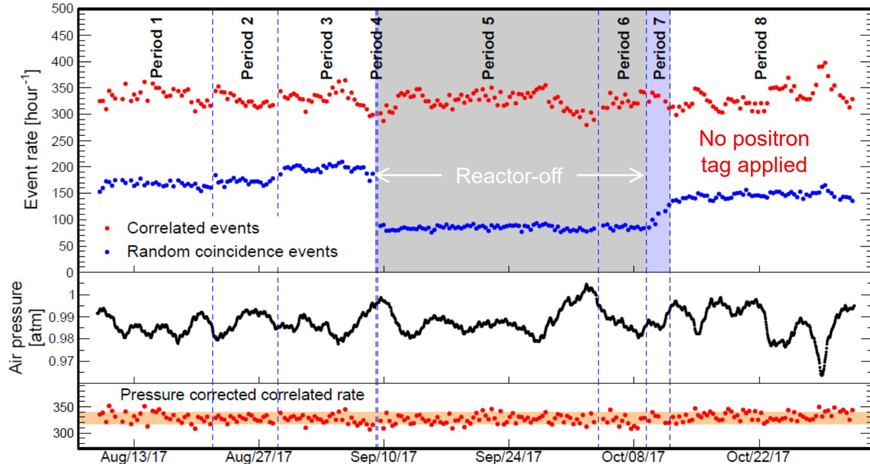
In this simple prototype, the positron tag improves the signal-to-noise by about a factor of five!
