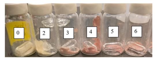
**Figure 5.** Ion-exchanged samples  $(45-90 \ \mu m)$  at different times of ion exchange in the increasing order of reaction time from 0 to 6 h.
