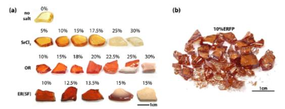
Figure 4. (a) Pictures of 78%TeO<sub>2</sub>-22%PbO glasses (mass basis) without salt (0%) and with varying amounts of SrCl<sub>2</sub>, oxide reduction (OR), and electrorefiner [ER(SF)] salt loadings—see ref 20 for more information. (b) Picture of 78%TeO<sub>2</sub>-22%PbO glass loaded with 10 mass% RECl<sub>3</sub> salt—see ref 21 for more information. All percentages listed are in mass%. Reprinted with permission from refs 20 and 21. Copyright 2017 and 2018 Elsevier.
