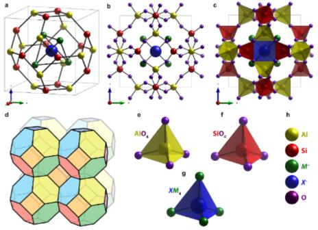
Fig.1 Sodalite  $\beta$ -cage shown in ball-stick format a without oxygen present, b with oxygen present, and e with oxygen and with space-filling polyhedra d a space-filling format with nine  $\beta$ -cages stacked together; tetrahedra including e AIO<sub>4</sub>, f SIO<sub>4</sub>, and g XM<sub>4</sub>; and h leg-
