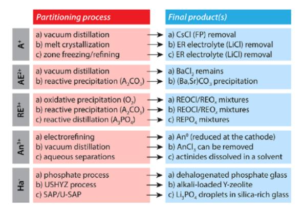
Figure 1. Summary of partitioning processes and final products targeting alkalis  $(A^+)$ , alkaline earths  $(AE^{2+})$ , rare earths  $(RE^{3+})$ , actinides  $(An^{3+})$ , and halides  $(Ha^-)$  where the product(s) listed are those resulting from the partitioning process. These are described in more detail in subsequent sections.
