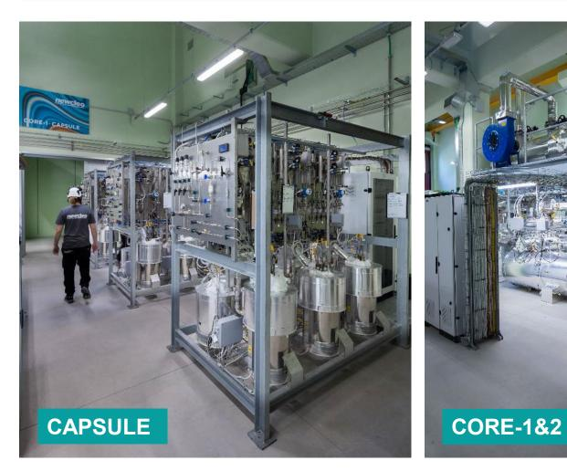
18 capsules for corrosion tests in stagnant lead, with advanced temperature and oxygen control
