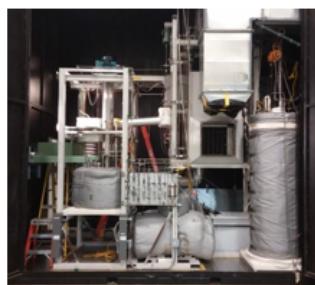
Liquid Salt Test Loop
