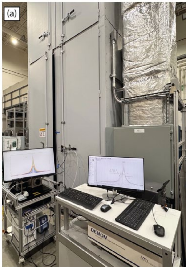
(a) FASTR storage tank with LIBS cart in the front left and DEMON spectrometer in the front right.
