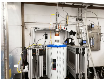
Setup for static corrosion experiments
