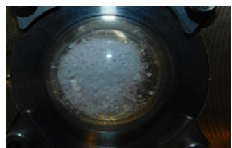
Custom hermetic sample holder to enable XRD measurements of molten salts under inert atmosphere
