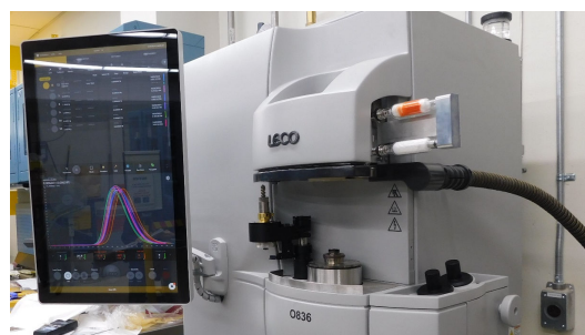
Inert Gas Fusion (IGF) for oxygen analysis (LECO O836)
