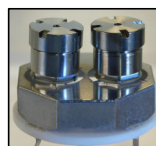
Modified CrNi with Ni liner tested and benchmarked using FLiNaK
