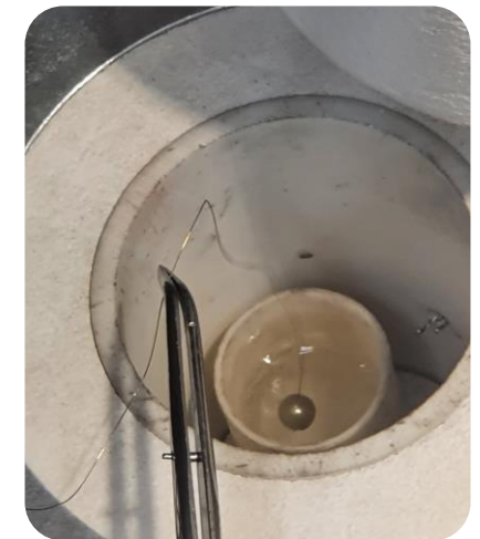
High T test with (Li,K)Cl eut. melt
