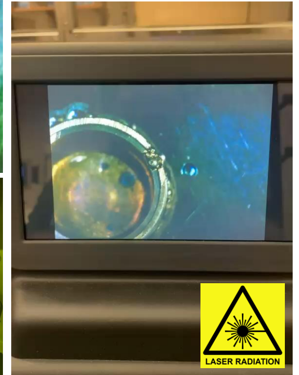
Laser welding Nd:YAG 1064 nm
