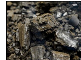
Crystallized NaCl- \text{UCl}_3 fuel salt (INL)
