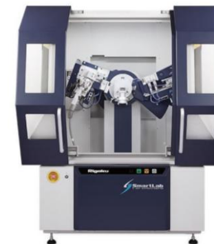
PXRD in transmission mode Prof. zur Loye group RT to 1100 °C
