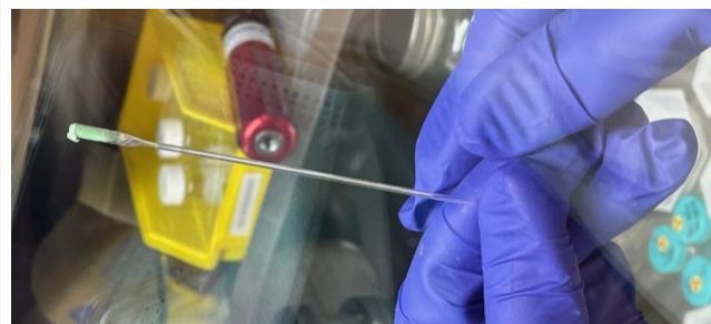
Sample sealed in fused silica capillaries
